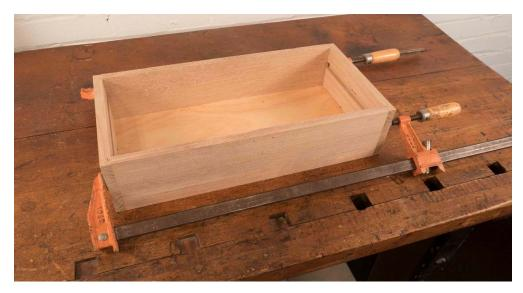
4) Locate, glue and install tray support rails in both the right and left sides. The supports should stay in place after pressing them in. If they move or fall out of the groove a couple pieces of masking tape can be used to hold them in place.
