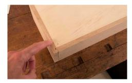
Check bottom flushness. This is to make sure the bottom is not in upside down.
