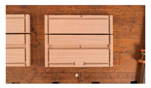
2) Lay the lower box parts on the table as shown. Note that the right side is to the right and the back is to the back and so on. The back is pre-drilled for hinges and the front is pre-drilled on center for the draw latch. The bottom of the box is the light-colored birch plywood. Add glue to the parts for assembly.
